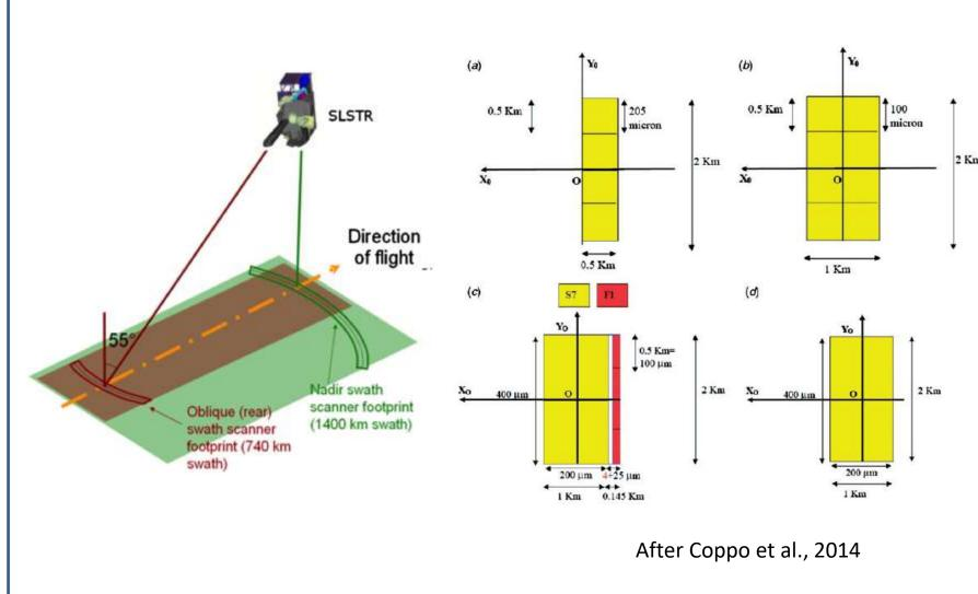
•The SLSTR scan has been optimized to allow a complete observation of the two BBs and the VIS calibration unit every two scans (0.6 sec) and the acquisition of both Earth views (near nadir and oblique) every scan (0.3 s).
